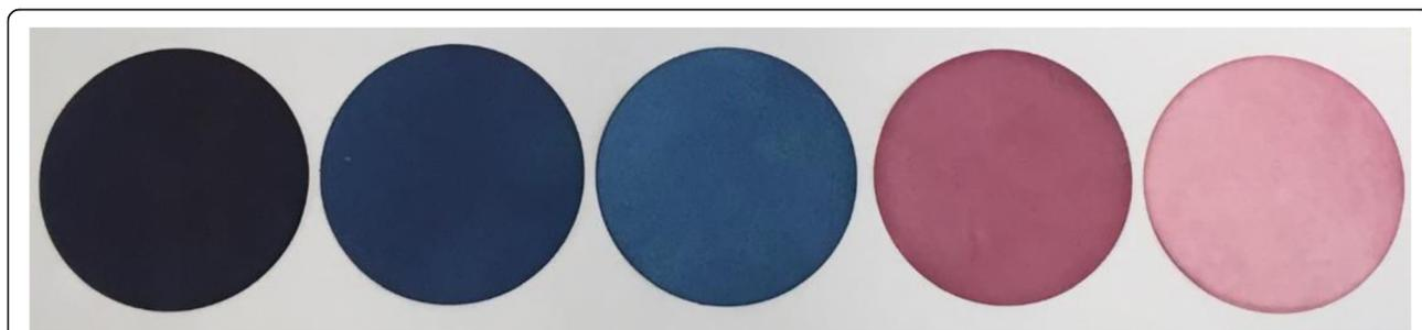
**Fig. 10** Photographs showing the color changes of probe **1** upon immersing in different concentration of  $\text{Ag}^+$  in HEPES solution (from left to right: 0.00, 0.05, 0.10, 0.50,  $1.00\ \mu\text{M}$ )
