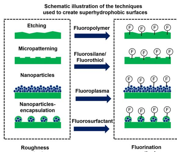
**Fig. 3** Schematic illustration of the techniques used to create superhydrophobic surfaces
