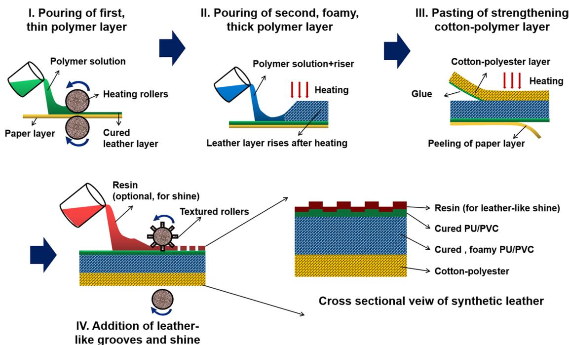
Fig. 1 Schematic representation of synthetic leather process
