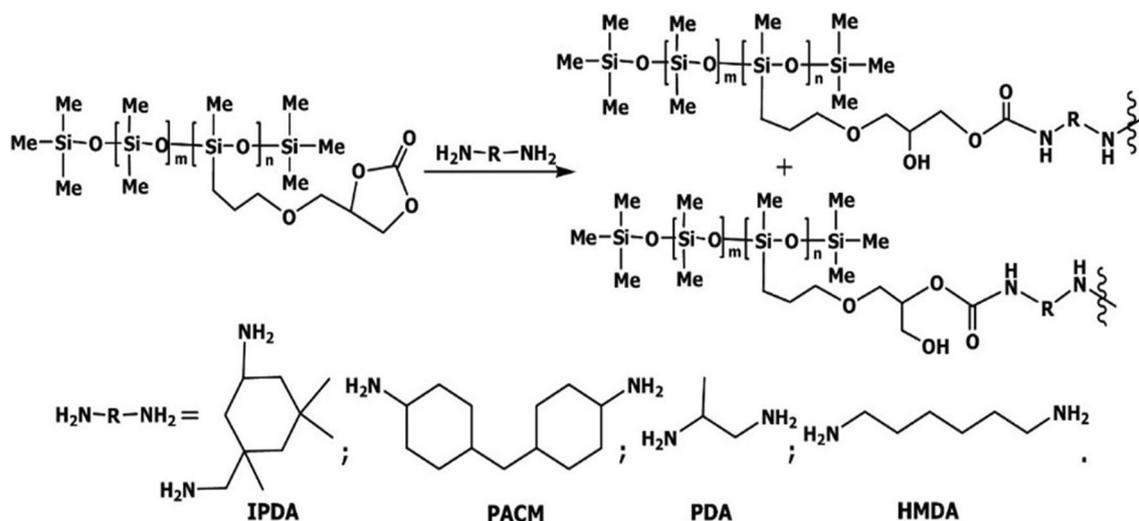
**Fig. 5** Synthetic routes of the NIPU coatings based on cyclic Polysiloxanes [63]. Copyright 2017, The Author(s), under the terms of the Creative Commons CC BY license
