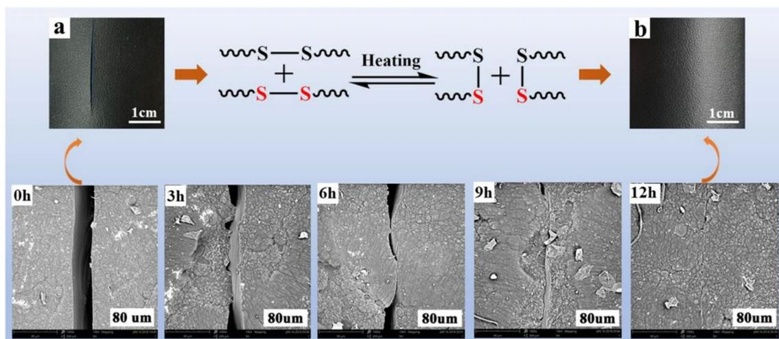
**Fig. 2** Self-healing process of leather coating: **a** damaged leather coating; **b** leather coating after be repaired at 60 °C for 12 h. SEM images show the self-healing process in time. Copyright 2020, The Author(s), under the terms of the Creative Commons CC BY license [60]
