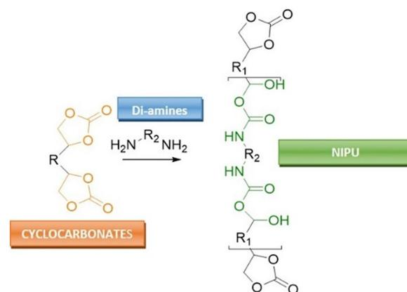
**Scheme 2** Non Isocyanate Polyurethanes (NIPUs) synthesis
