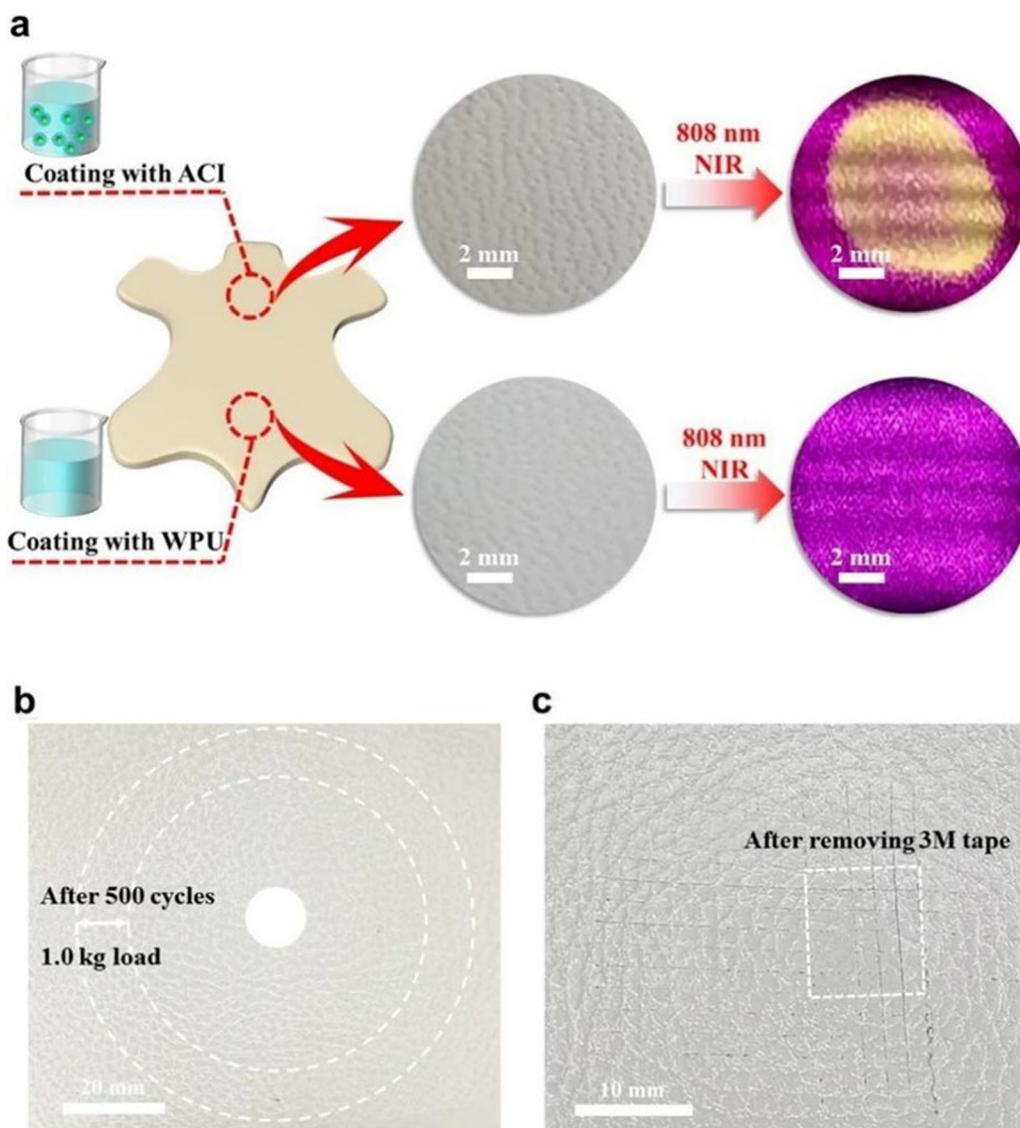
**Fig. 4** a Naked eye observations of patterns under 808 nm NIR laser excitation of invisible anti-counterfeiting leather products. The digital images show ACLs after the abrasion test (b) and adhesive peel strength test (c) on the leather products. Scale bars = 20 mm (a) and 10 mm (b). Copyright 2021, The Author(s), under the terms of the Creative Commons CC BY license [81]
